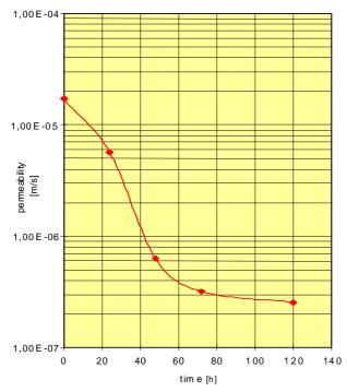
Permeability reduction of a sandstone Fig. 4: sample during treatment with CaSO<sub>4</sub> supersaturated solutions
