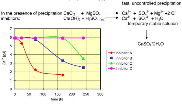
Fig. 1: Course of gypsum crystallizationdepending on the inhibitor used
