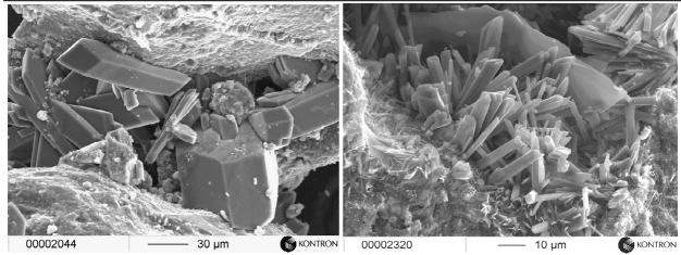
Fig. 2: Flow paths sealed by gypsum crystals Fig. 3: Gypsum needles covering the surface
