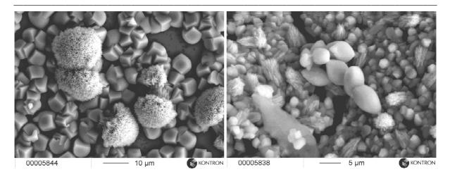
Fig. 2, 3: SEM of different CaCO<sub>3</sub> crystals covering a mineral surface
