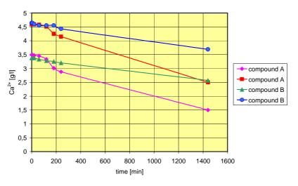
Fig. 1: Course of CaCO<sub>3</sub> precipitation depending on the used carbonate releasing compound
