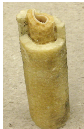
Growing crust resulting from supersaturated \text{CaSO}_4 - solution
